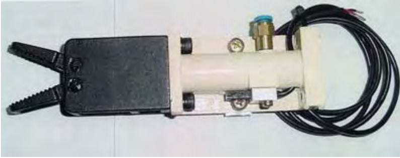
# TOP10022 NARROW GRIPPER FOR SHORT SPRUE
